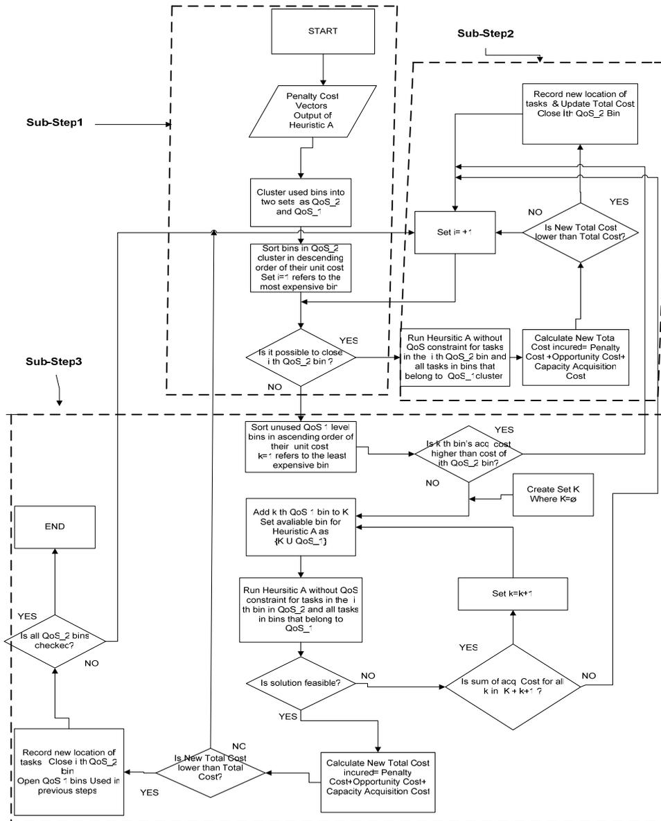
Figure 1: The Flowchart of Proposed Heuristic
